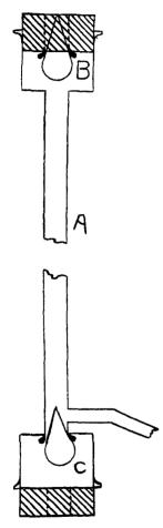
the lower part of the inner cylinder and is entirely immersed in the acid of the reservoir. At each end is a floating glass valve playing upon a rubber cushion at the end of the tube. When the gas is turned on and the pressure relieved from the inner cylinder the acid can enter only at B, and when the action is reversed the acid can escape only at C.
